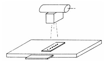
Figure 2-1. Diagram Showing Arrangement of Grid Alignment Test Tool for Checking Grid Alignment
